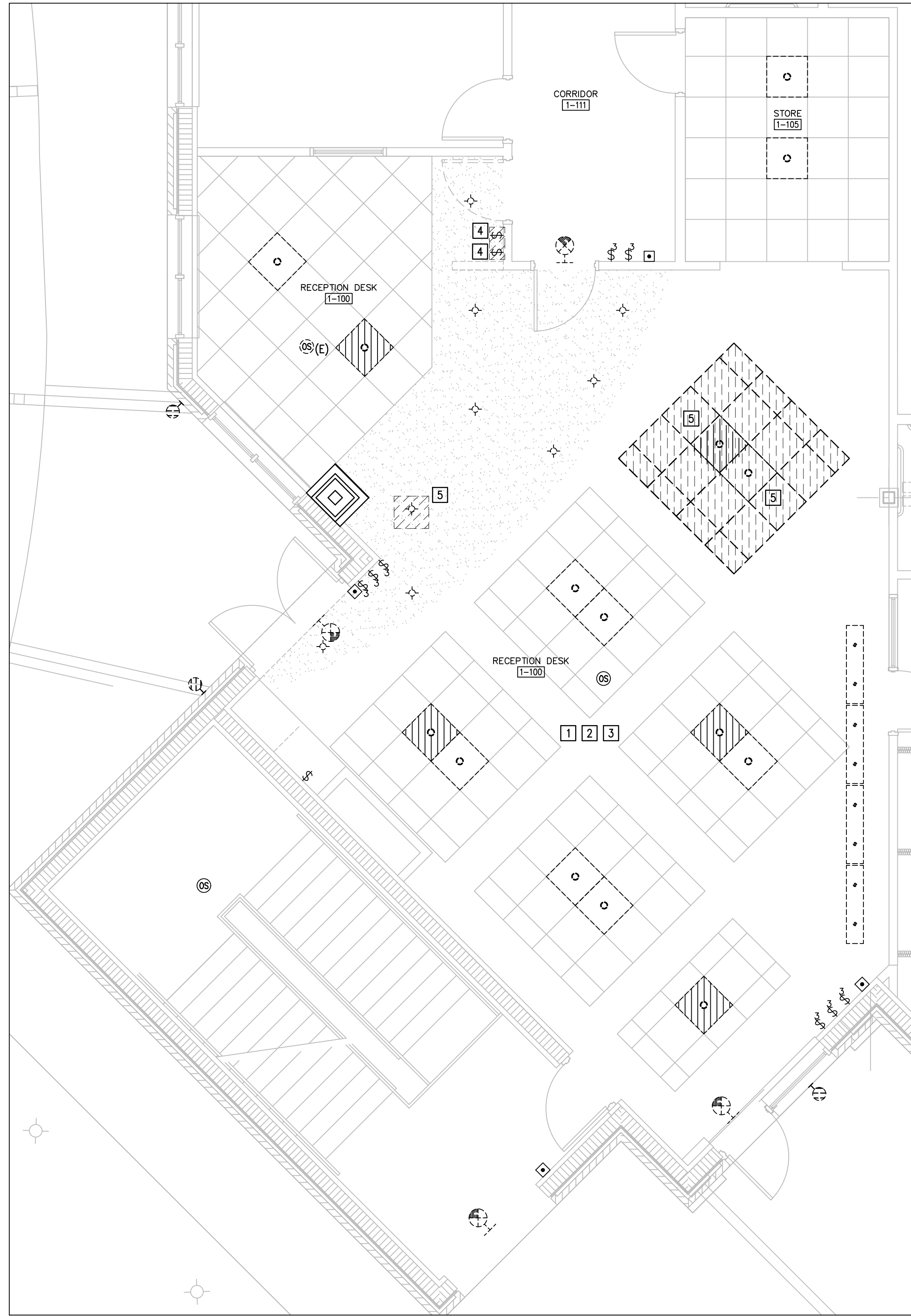
1 LIGHTING PLAN - DEMOLITION 1 2 3 SCALE: 1/4" = 1'-0"
