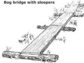
Figure 50-A simple bog bridge with sleepers. This common structure is also called a single-plank boardwalk in coastal Alaska.
