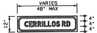
W16-8B-XX MOUNTED BELOW 36" W2 OR W3 WARNING SIGN NOTE: LETTER TYPE AS APPROPRIATE (TYPE C OR D) B/FY, RB
