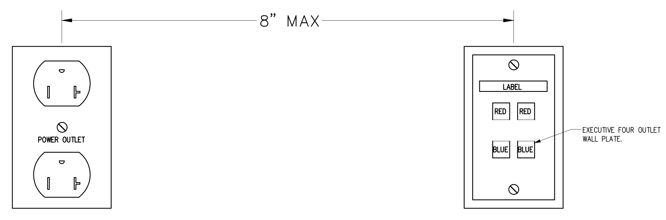
1 TYPICAL OUTLET CONFIGURATION ES6.1 SCALE: FULL SIZE THE CONTRACTOR SHALL COORDINATE THE POWER AND PHONE/DATE OUTLETS SHOWN ON THE TWO SETS OF DRAWINGS. WHERE DEVICES ARE SHOWN ON THE SAME WALL THEY SHALL BE INSTALLED AS SHOWN ABOVE. THIS APPLIES TO THE JAIL AND COURT BUILDINGS.
