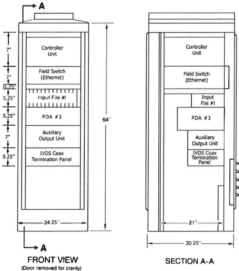
Figure 925-1 Typical 334 Cabinet Configuration
