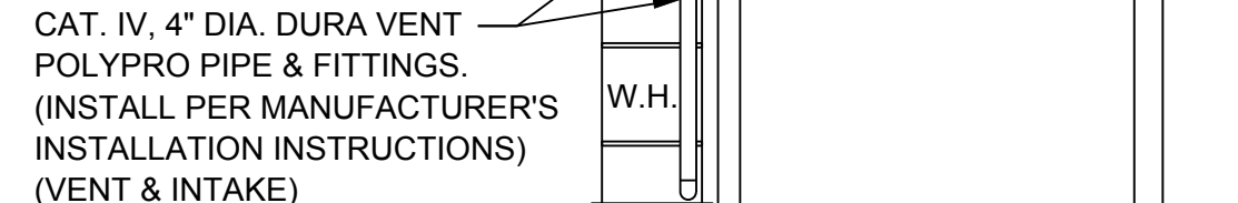
6 WATER HEATER VENT & FRESH AIR INTAKE M42 SCALE: NONE
