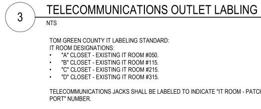
OUTLET JACKS TO WHICH THEY ARE CONNECTED. PATCH PANELS SHALL BE LABELED IN ALPHABETICAL ORDER FROM TOP TO BOTTOM / PORTS LABELED LEFT TO RIGHT FOR EACH PATCH PANEL. CABLING: EACH CAT. 6 CABLE SHALL BE LABELED 12 INCHES FROM EACH TERMINATED END WITH "IT ROOM -PATCH PANEL - JACK/PATCH PANEL PORT" NUMBER.
