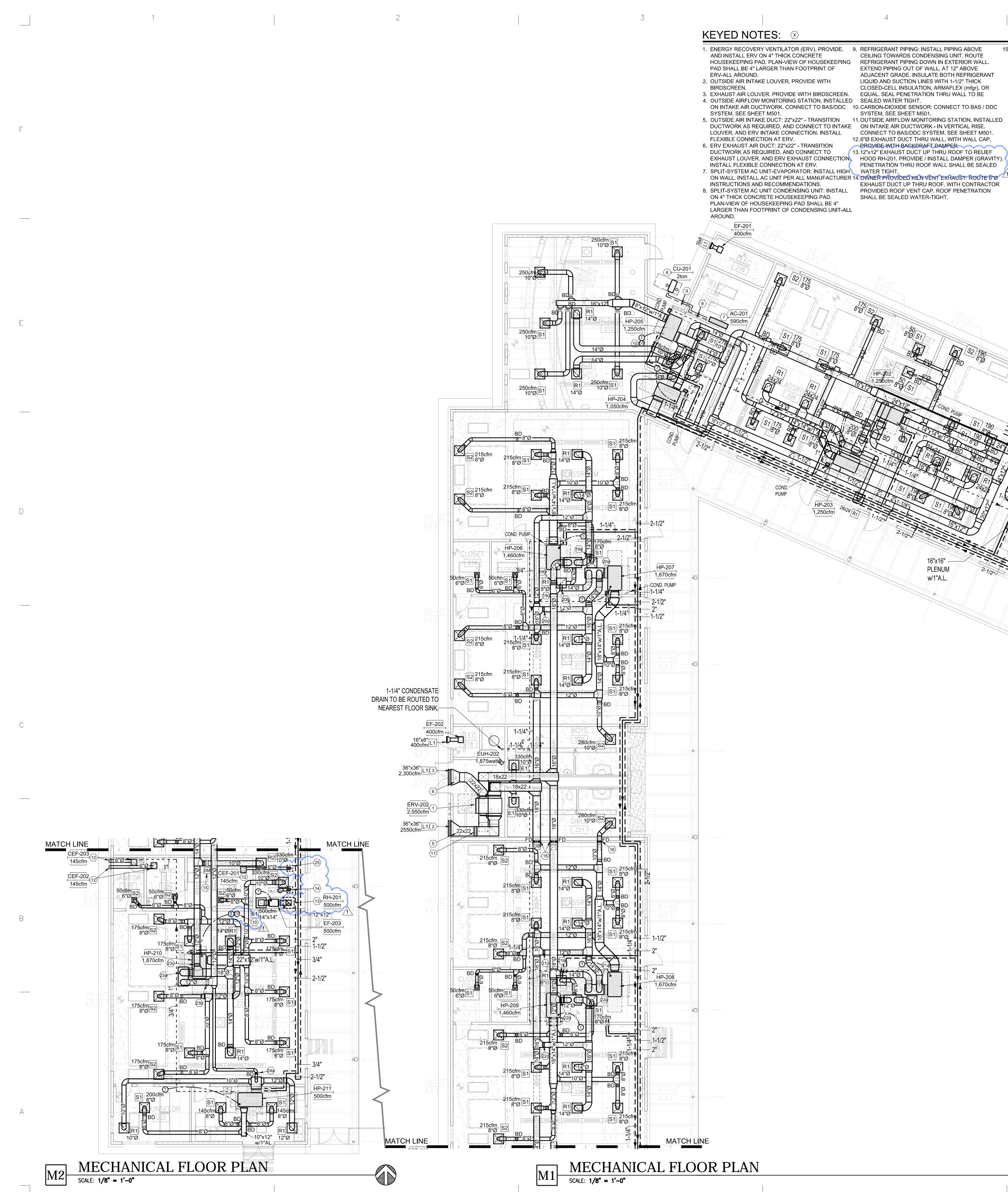
15. OPERATION OF KILN ROOM [227]: INSTALL MOTORIZED DAMPER IN EXHAUST DUCT AT DOOR. CONNECTED TO ERV-202 EXHAUST. SEQUENCE OF OPERATION(S): a. NORMAL OPERATION OF KILN ROOM [227]: -- KILN EQUIPMENT IS ENABLED "OFF". - SUPPLY AIR TO KILN ROOM IS SUPPLIED AT 330CFM (from HP-210). - MOTORIZED DAMPER IN EXHAUST DUCT SHALL ROOM SHALL T&B'd TO BE 350CFM, (PROVIDES 6% NEGATIVE PRESSURE).
