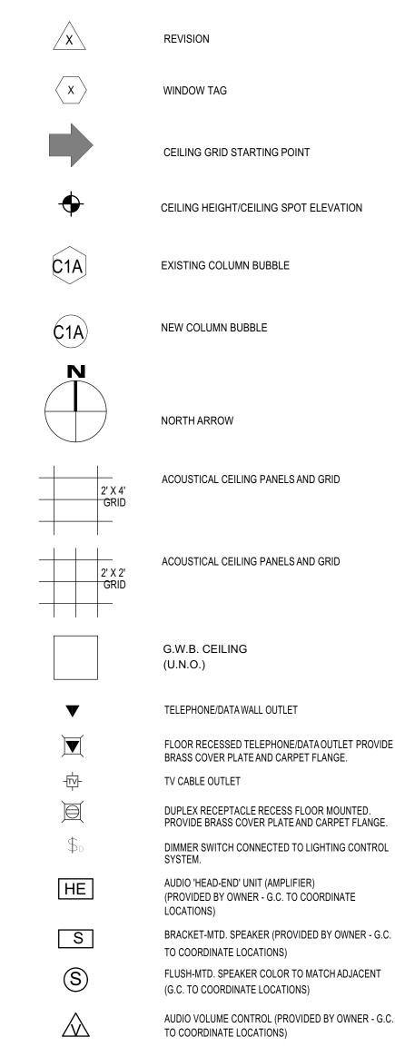
(PROVIDED BY OWNER - G.C. TO COORDINATE BRACKET-MTD. SPEAKER (PROVIDED BY OWNER - G.C. FLUSH-MTD. SPEAKER COLOR TO MATCH ADJACENT AUDIO VOLUME CONTROL (PROVIDED BY OWNER - G.C. WALL-MTD. MICROPHONE JACK (PROVIDED BY OWNER -G.C. TO COORDINATE LOCATIONS) CEILING MOUNTED CAMERA, BY OWNER (G.C. TO COORDINATE LOCATIONS) WALL MOUNTED CAMERA, BY OWNER (G.C. TO COORDINATE LOCATIONS)
