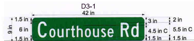
TYPICAL STREET SIGN FACE DETAIL
