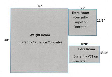
Multipurpose room shall receive Resilient Taraflex Multi-Use 6.2 flooring or "approved equal".
