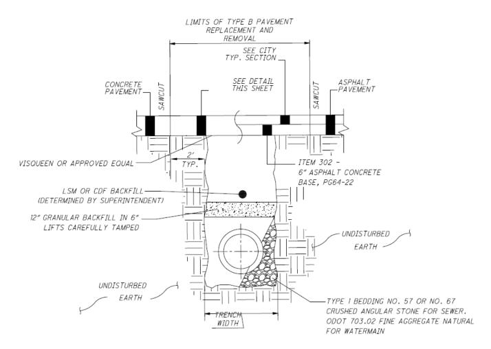
15. Any settlement in open trench backfill taking place within guaranteed period shall be refilled with satisfactory materials & affected surface properly repaired by contractor at the expense of the contractor at no additional cost to the city
