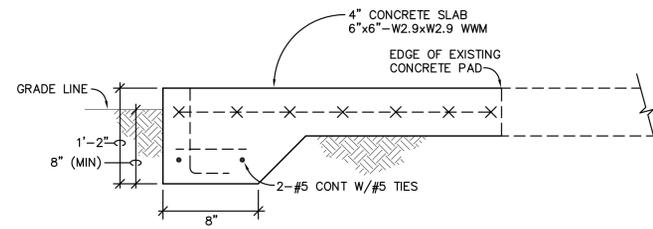
**SECTION AT CONDENSING UNIT PAD**
