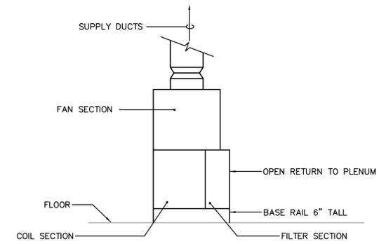
**TYPICAL AIR HANDLING UNIT DETAIL**
