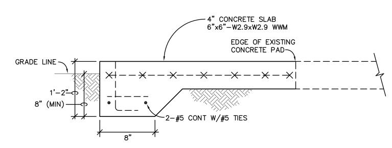
SECTION AT CONDENSING UNIT PAD
