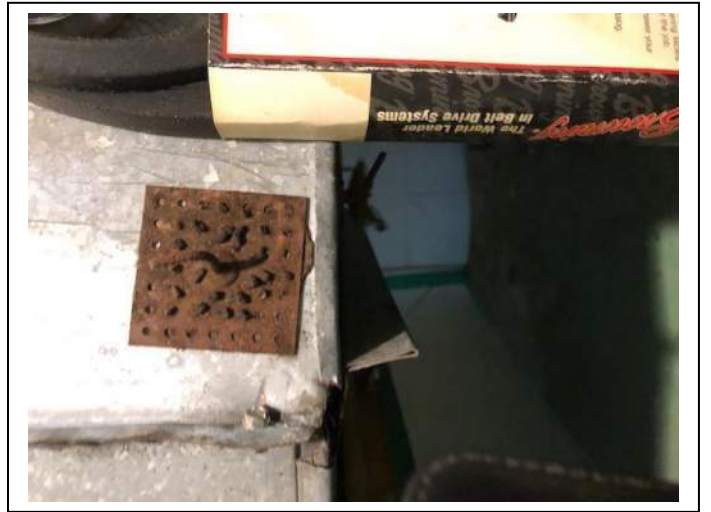
Photo #12 Material: Brown Pin Mastic Sample Result: 40% Chrysotile
