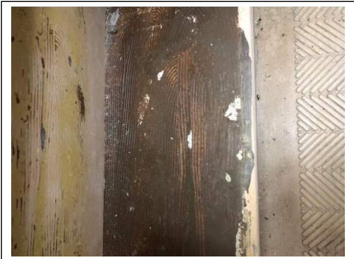
Photo #11 Material: Sample Result: Brown Stair Tread Mastic Sample Result: No Asbestos Detected
