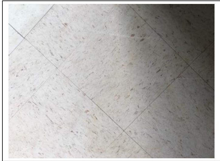
Photo #52 Material: 12"x12" White With Pink Specks Floor Tile Sample Result: No Asbestos Detected
