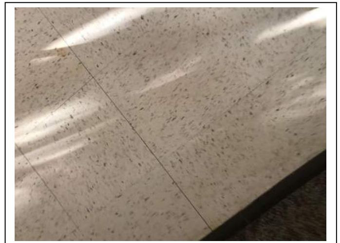
Photo #28 Material: 12"x12" White With Black Specks Floor Tile Sample Result: No Asbestos Detected
