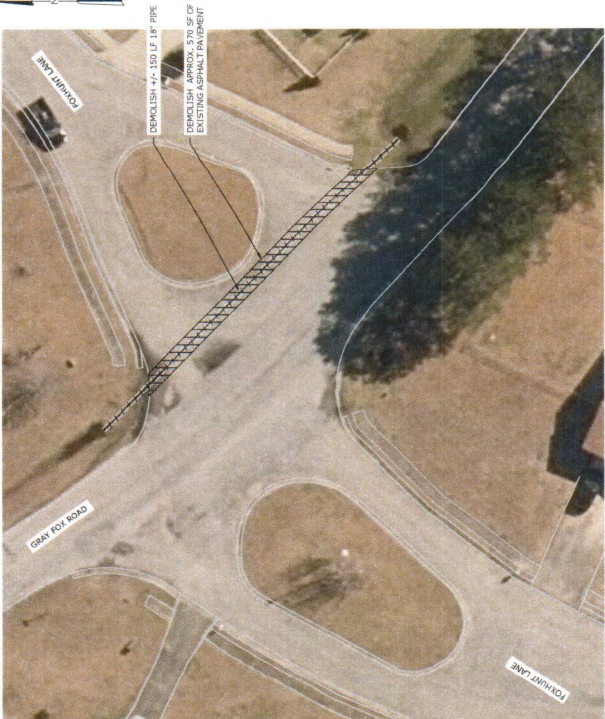
DEMOLITION PLAN SCALE: 1" = 20'
