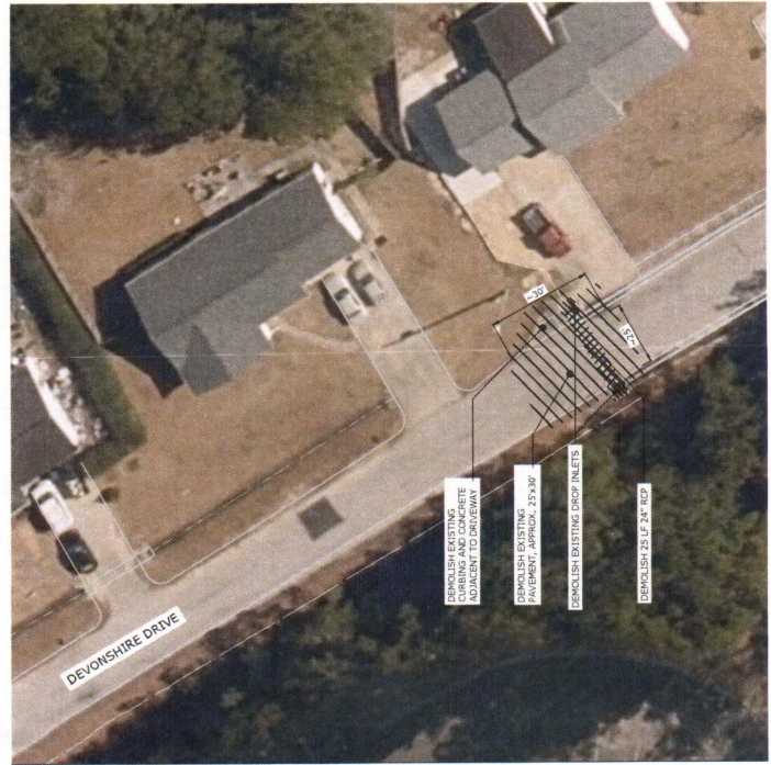
DEMOLITION PLAN SCALE: 1" = 20'
