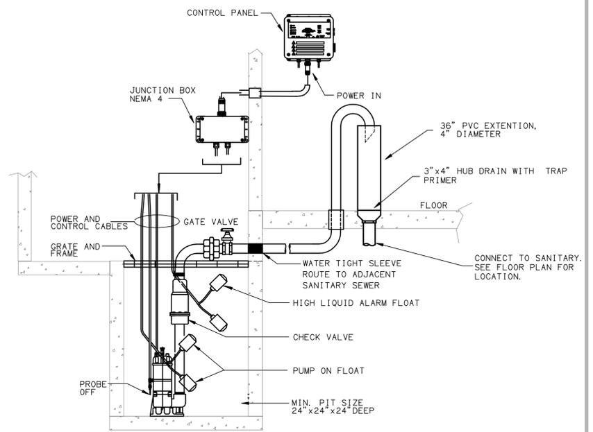
OIL MINDER SUBMERSIBLE SUMP PUMP PACKAGE SYSTEM- STANCOR MODEL NO. SE-50; .5 HP, 115V, 3600 RPM, 2" DIA. DISC., JUNCTION BOX, CONTROL PANEL W/ AUDIBLE AND VISUAL ALARM, SILENCING SWITCH, DRY CONTACTS FOR REMOTE MONITORING, POWER CABLE, CONTROL CABLES, LIGHTS FOR OIL SPILL, POWER, HIGH LIQUID LEVEL, OVERLOAD AND PUMP RUN. SYSTEM SHALL BE A COMPLETE PACKAGE.
