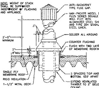
**FLUE THRU ROOF DETAIL 10**
