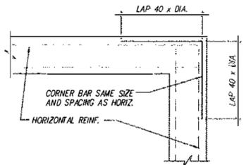
1 TYPICAL CORNER AT CONCRETE FOOTINGS AND WALLS
