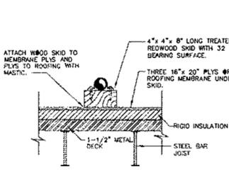
**ROOF PIPING SUPPORT DETAIL**
