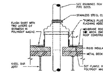
**PIPE PENETRATION THRU ROOF DETAIL**
