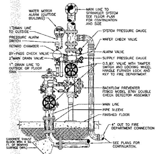
**WET PIPE FIRE RISER DETAIL 1**
