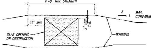
13 TYP. TENDON LAYOUT AT OPENINGS OR OBSTRUCTIONS - PLAN VIEW
