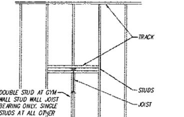
16 TYP. JOIST BEARING DETAIL
