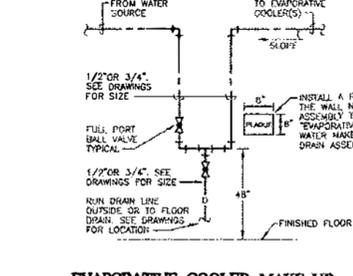
**EVAPORATIVE COOLER MAKE-UP AND DRAIN ASSEMBLY**
