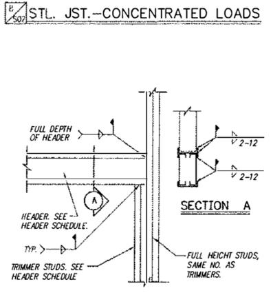
9 TYPICAL HEADER BEARING DETAIL
