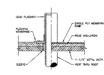
**VENT THRU ROOF DETAIL**
