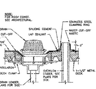
**ROOF DRAIN DETAIL**
