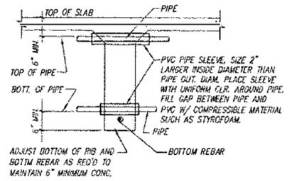
14 TYP. DETAIL AT PIPE PENETRATION THROUGH P/T SLAB RIB
