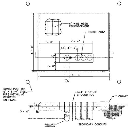
**THREE PHASE RADIAL FEED TRANSFORMER PAD DETAIL**
