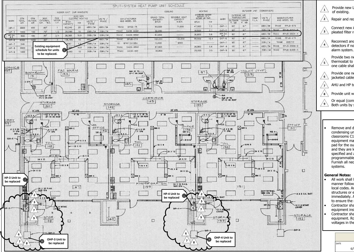
Provide new LON thermostat Viconics part # VT7600H55E or equal in place
