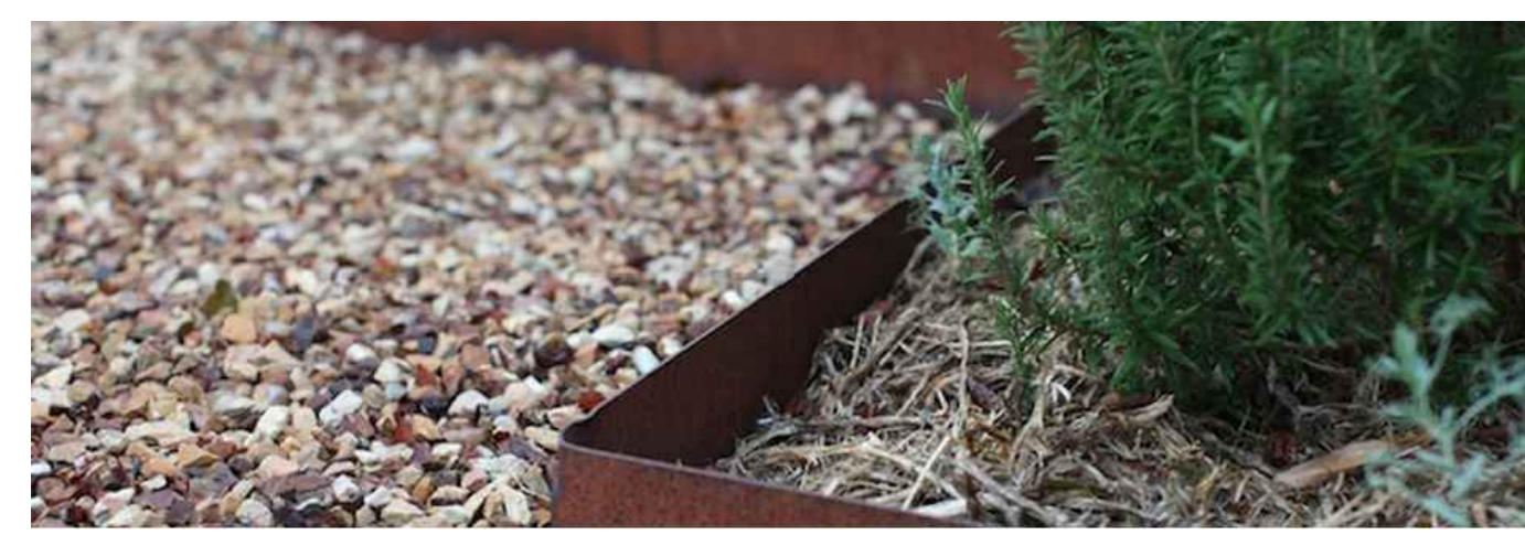
9 CORTEN METAL EDGING EXAMPLE IMAGE L-0302 SCALE: NTS MATERIAL: CORTEN STEEL WIDTH: 4" -INSTALL EDGING AT BOUNDARY OF ALL LANDSCAPE BEDS
