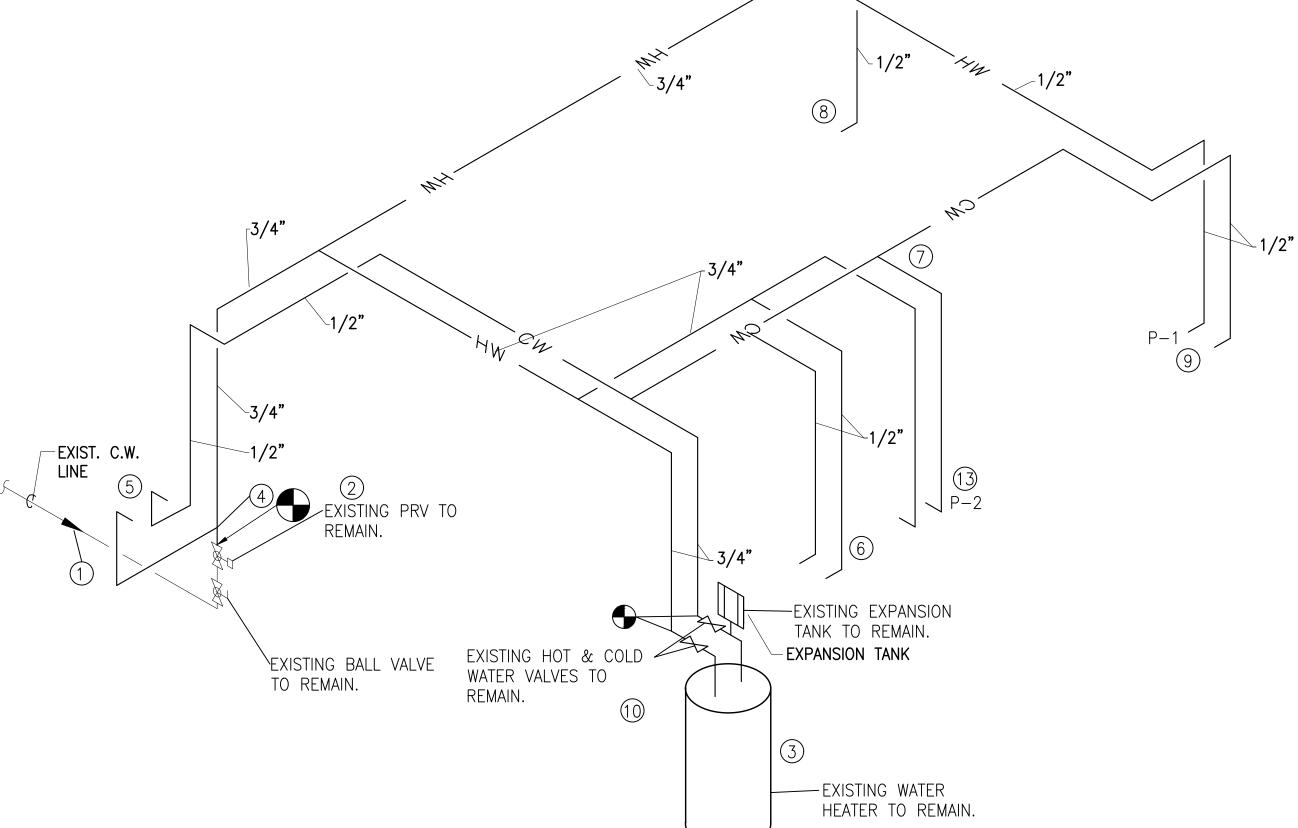
FIRST FLOOR ACCESSIBLE - WATER RISER DIAGRAM - BUILDING A SCALE: (OTHER SIDE MIRRORED)
