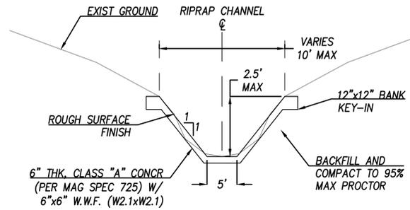
**D** CONCRETE CHANNEL CROSS SECTION
