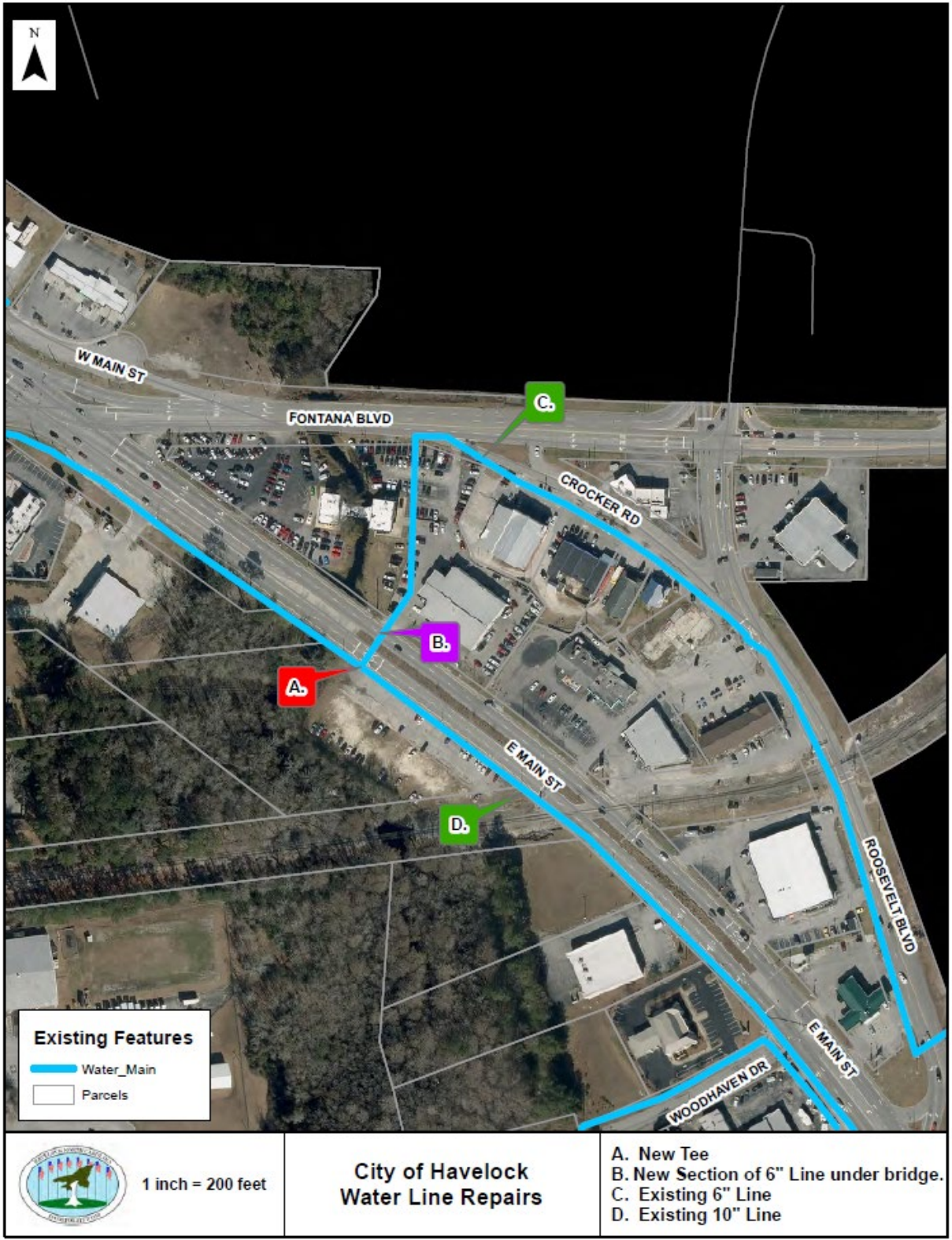
Figure 1a MAP: PIPE REPLACEMENT
