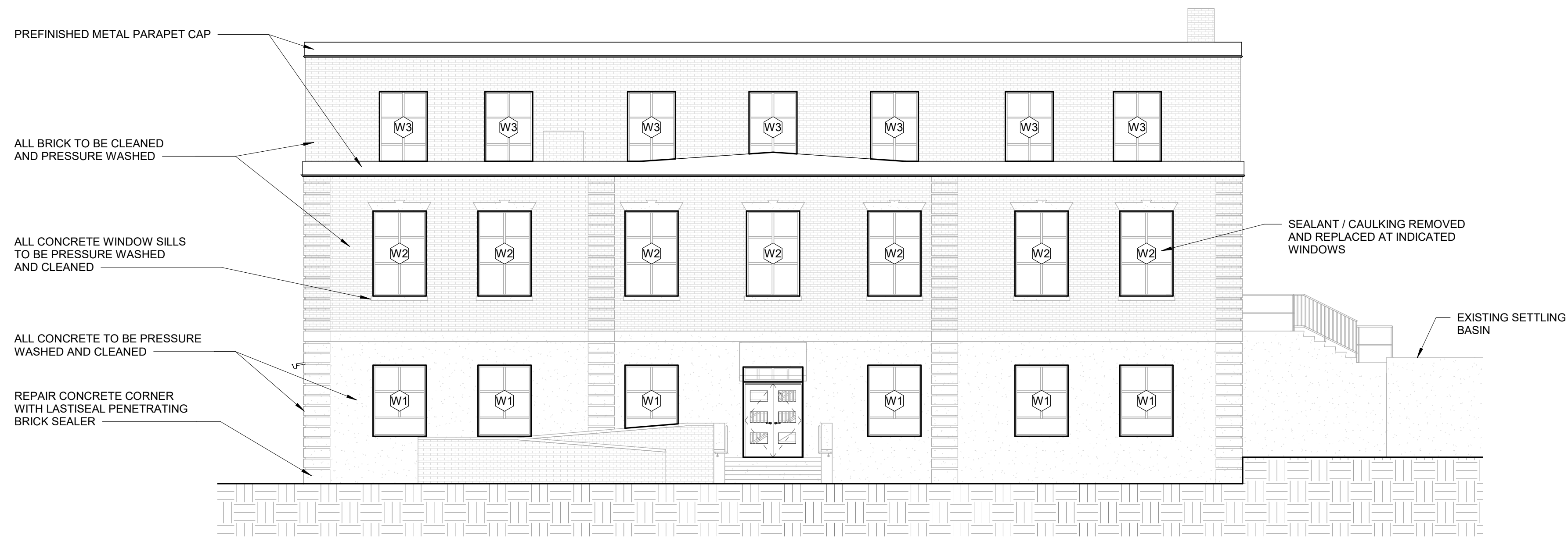
1 FILTER BUILDING ELEVATION 49-A202 SCALE: 1/8" = 1'-0"
