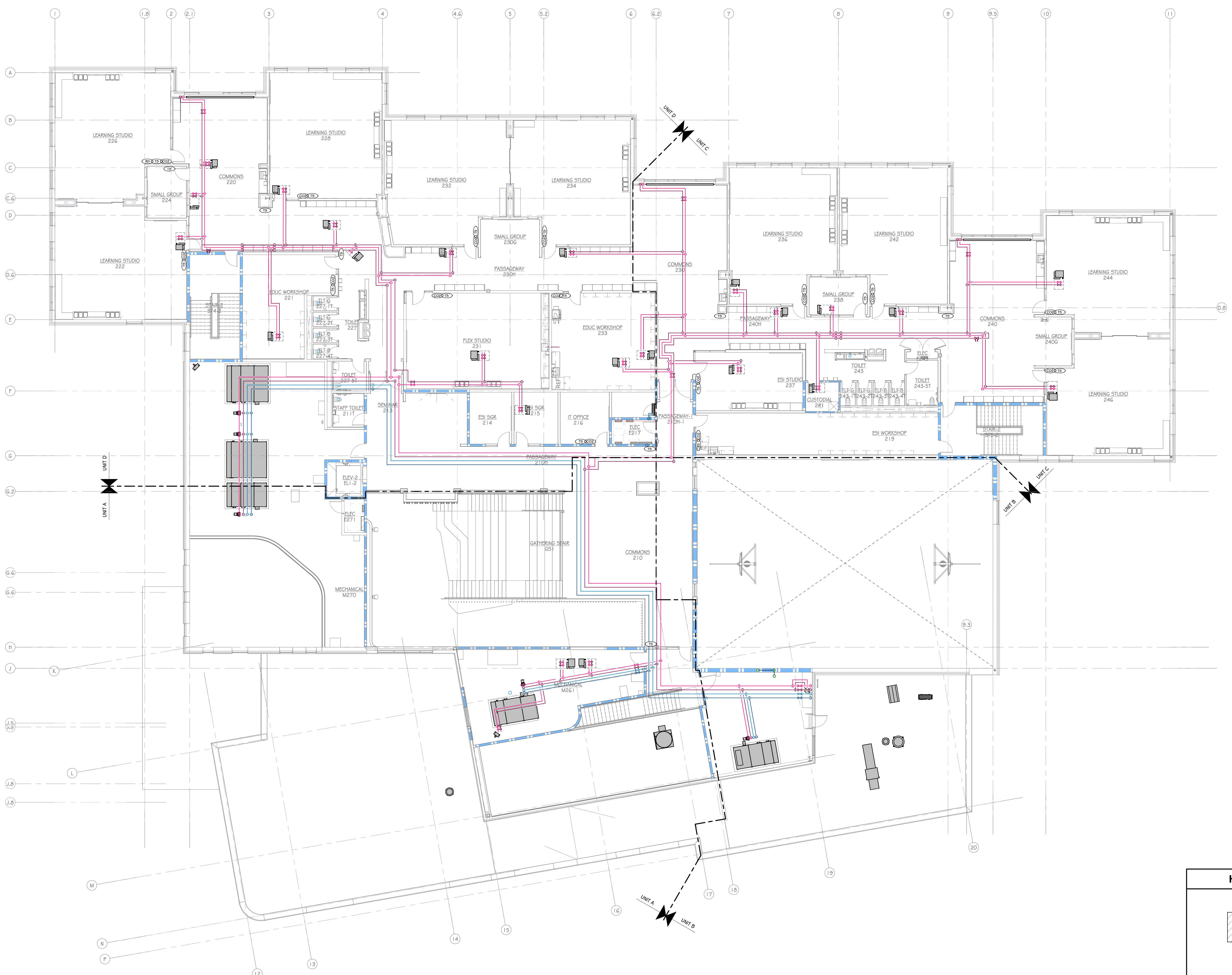
SECOND FLOOR HVAC PIPING PLAN - OVERALL 1" = 10'-0"
