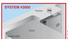
System #3000 consists of: #328 ( hinge side ) #326 ( head & lock sides )
