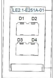
**Figure 2** – Acceptable substitute labeling method for non-Laney projects.
