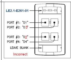
**Figure 3 -** Incorrect progression: Port numbers should not progress down columns.
