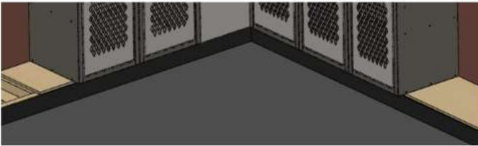
Figure E – Complete all the tops and secure the bases to the floor
