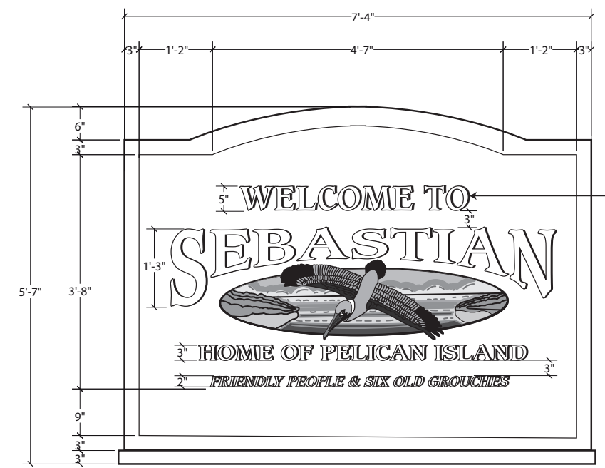
Sign Face - Detail Scale 1/2in = 1ft
