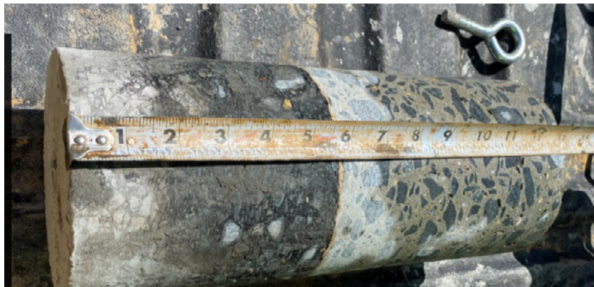
TOP Surface Course Base Course Concrete BOTTOM
