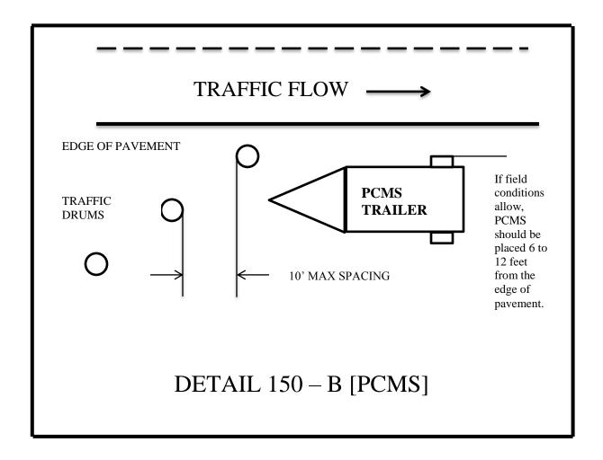
When not in use, the PCMS shall be removed from the roadway, unless protected by positive barrier protection. If the PCMS is protected by positive barrier protection, the sign panel shall be turned away from traffic when not in use.
