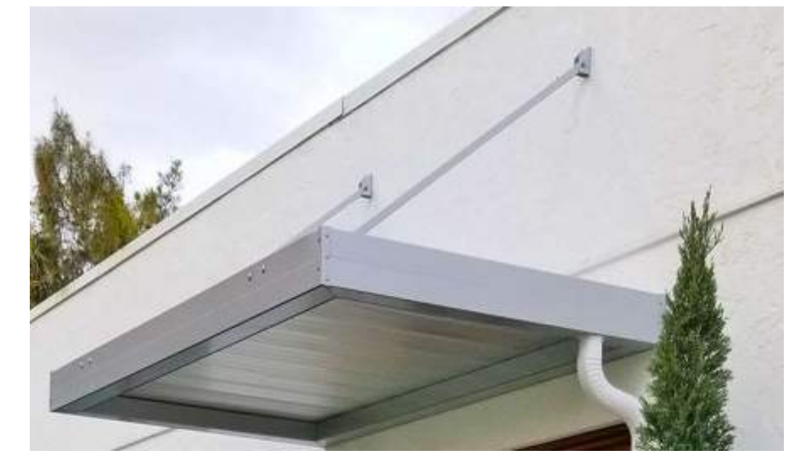
80" WIDE X 60" PROJECTION IMPERIAL MARQUEE ALUMINUM AWNING WITH 8" WIDE FLAT PANELS, SQUARE TUBING OVERHEAD BRACES, EXTRUDED ALUMINUM 6" TALL GUTTER AND DOWNSPOUT KIT AS MANUFACTURED BY GENERAL AWNINGS, LLC OR APPROVED EQUAL (POWDERCOATED COLOR TO BE SELECTED BY OWNER)
