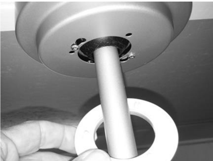
Photo 7: Key holes on the bottom of the hanger cover.
