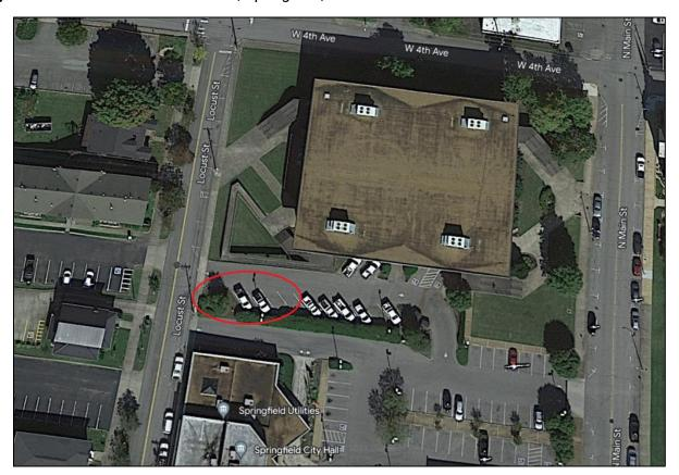
**Project Scope** - Project consists of the site work and electrical activities to facilitate the installation of paired ChargePoint Express 250 equipment to provide up to 125kW of rapid electric vehicle charging capability. The installation and activation of the EV charging equipment is not included in this scope of work; however, the EV charger footprint template will be provided by the owner for anchor bolt and electrical conduit layout and installation by the awarded bidder.
