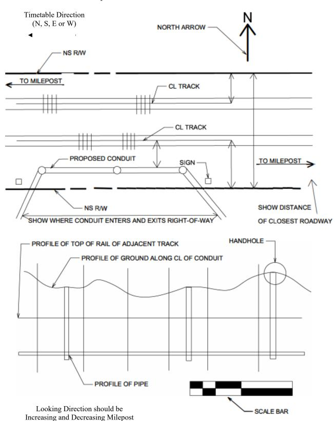
Plate IX - Sample Conduit Parallel Section View
