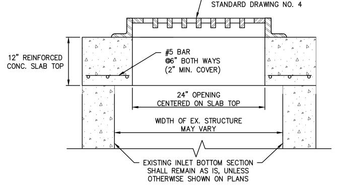
SIDE VIEW INLET RECONSTRUCTED TO GRADE, AS PER PLAN (FLAT TOP)
