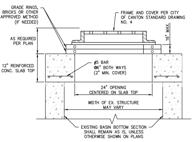
SIDE VIEW INLET RECONSTRUCTED TO GRADE, AS PER PLAN
