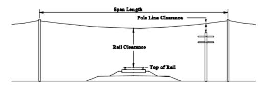
In no case shall crossings have less vertical clearance than the following at a final unloaded sag at 60° F, or for span lengths greater than the standard span lengths for the appropriate geographic loading district, at the maximum conductor temperature for which the supply line is designed to operate.
