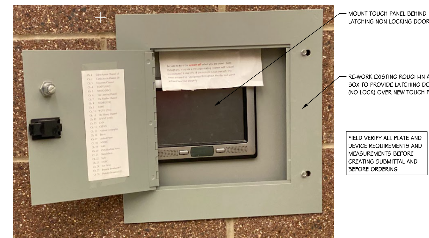
CHS COMMONS "TP" TOUCH PANEL DETAIL SCALE: NONE
