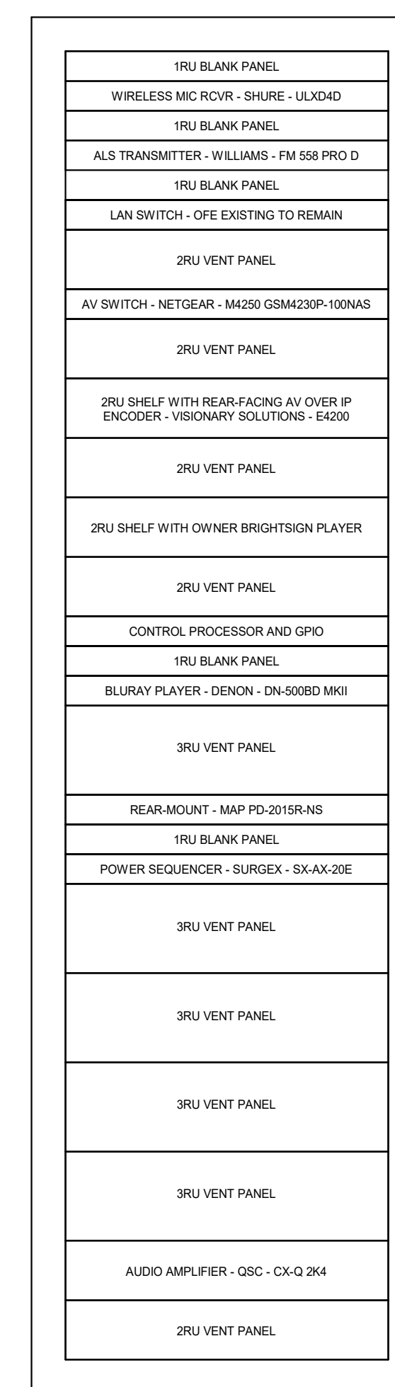
CHS COMMONS RACK ELEVATION DETAIL 1/12" = 1'-0"
