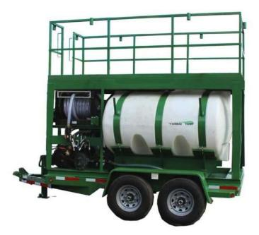
The HM-1000-HARV, is a 1000 gallon hydroseeder with mechanical (paddle) agitation. It is available as both a skid type and a pull type system. It will seed 13000 square feet per load. It is equipped with an 27 H. P. Kohler Command Pro electric start engine, a hydraulically driven paddle agitation that is reversible and also has adjustable speed. It has a hydraulically driven reversible Bowie gear pump.
