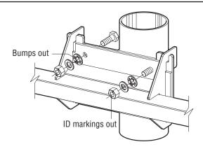
Snug all nuts. Using supplied 1½ in wrench, tighten each nut until plates are in firm contact. Follow tightening sequence shown.
