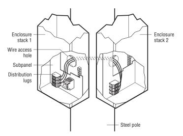
Connect equipment grounding conductors (green/yellow) from each upper enclosure to equipment ground bar in bottom enclosure. If pole has multiple stacks, connect bonding jumper from stack one.
