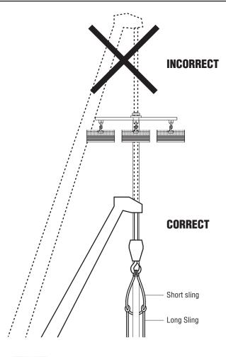
When pole is suspended, insert rotator bar to clamp and turn to lock in place. Guide pole into position over base using rotator bar and lower onto base. Do not allow pole to seat on base until it is properly aimed (step 9). Pole should rotate with reasonable force applied to bar, but not freely.
