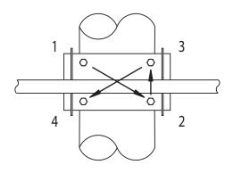
Using supplied breaker bar, 11/16 in socket, extension, and wrench, tighten each nut until orange extrusion appears from at least three bumps.
