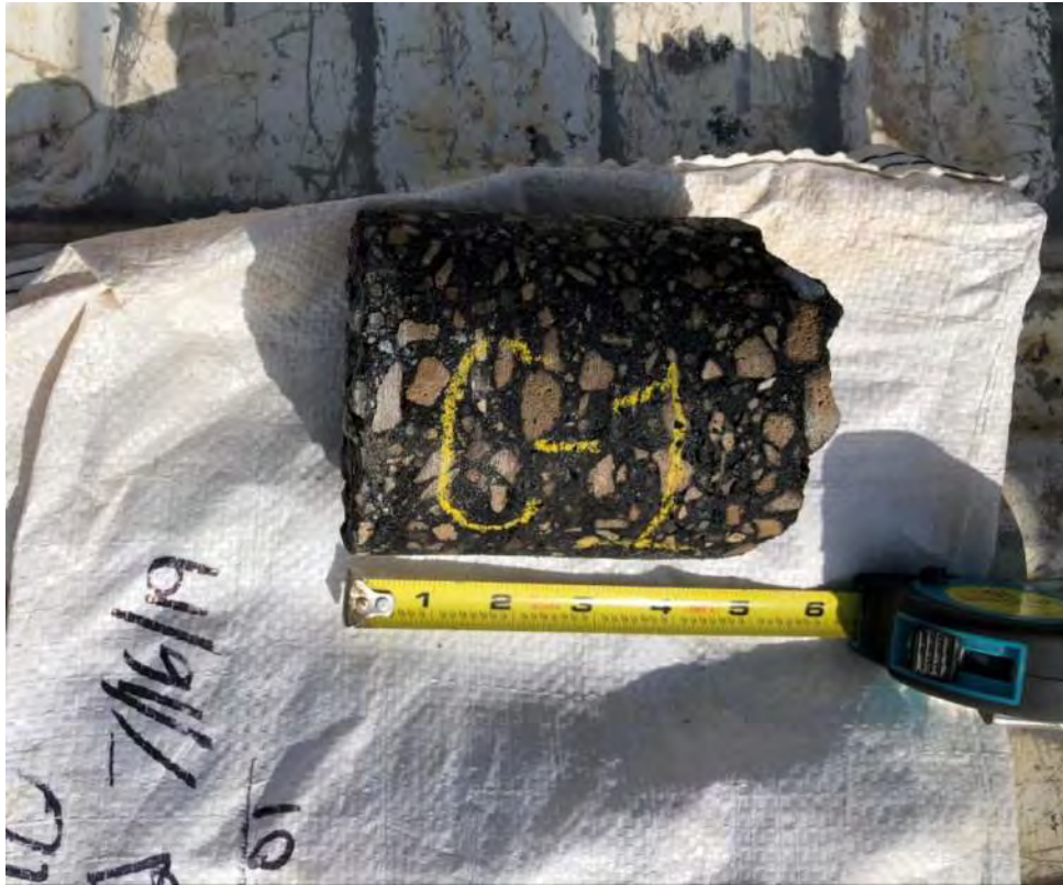
Core C-1 - Approximately 5¼ Inches of Asphaltic Concrete
