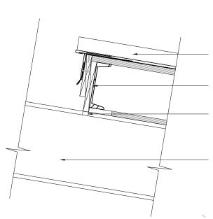
STANDING SEAM METAL ROOFING OVER ROOFING MEMBRANE OVER 5/8" CDX PLYWOOD OVER ROOF FRAMING
