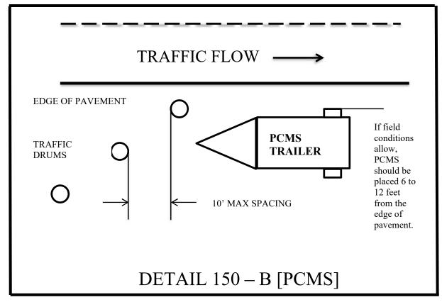
When not in use, the PCMS shall be removed from the roadway, unless protected by positive barrier protection. If the PCMS is protected by positive barrier protection, the sign panel shall be turned away from traffic when not in use.
