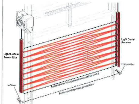
Image shows infrared beam pattern which is not visible to the naked eye.
