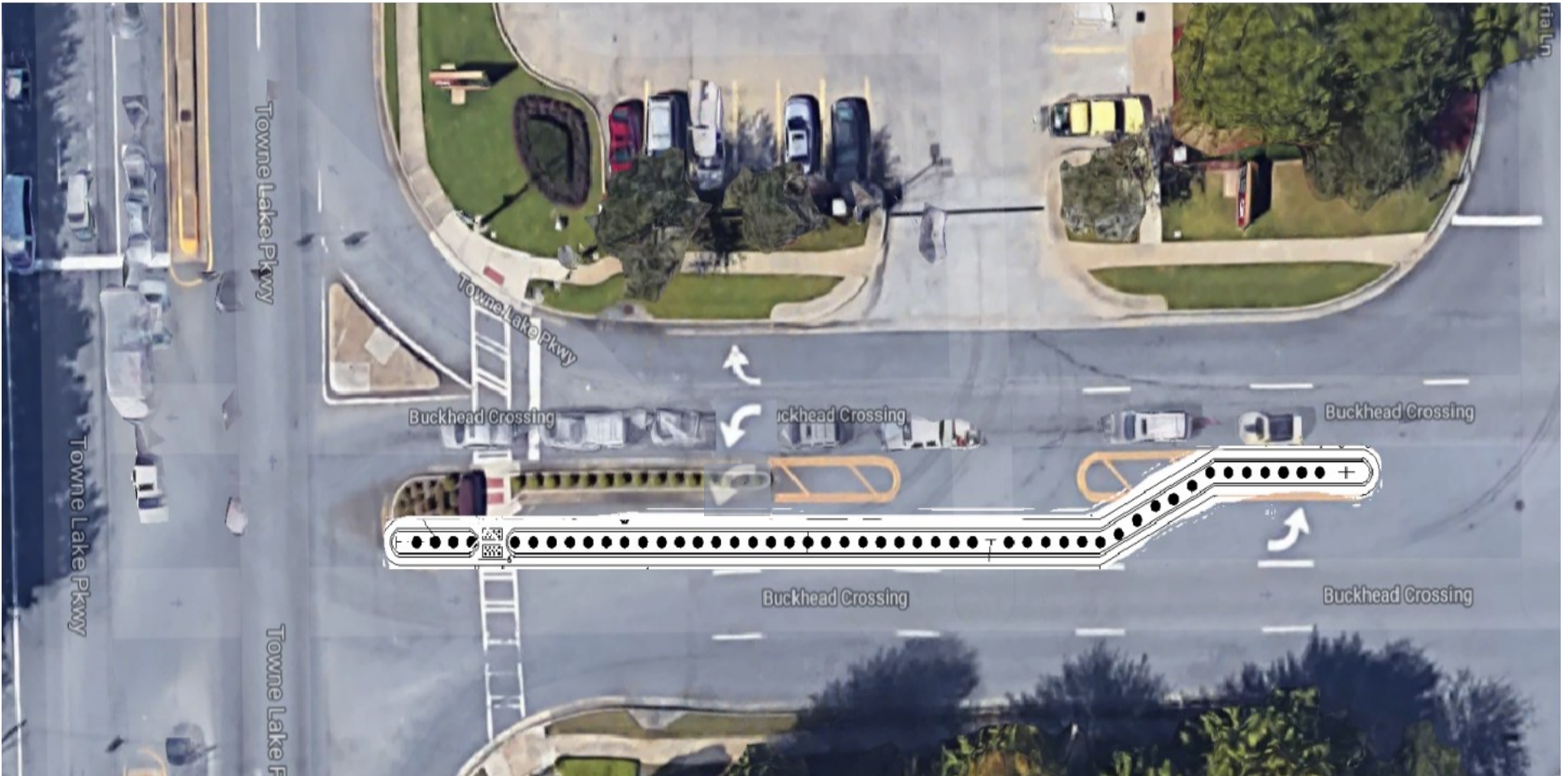
Construction Reference Line—showing pavement demolition and sawcut line.
