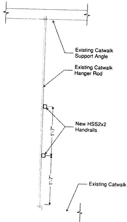
Figure 2a: Replace handrails with square HSS members
