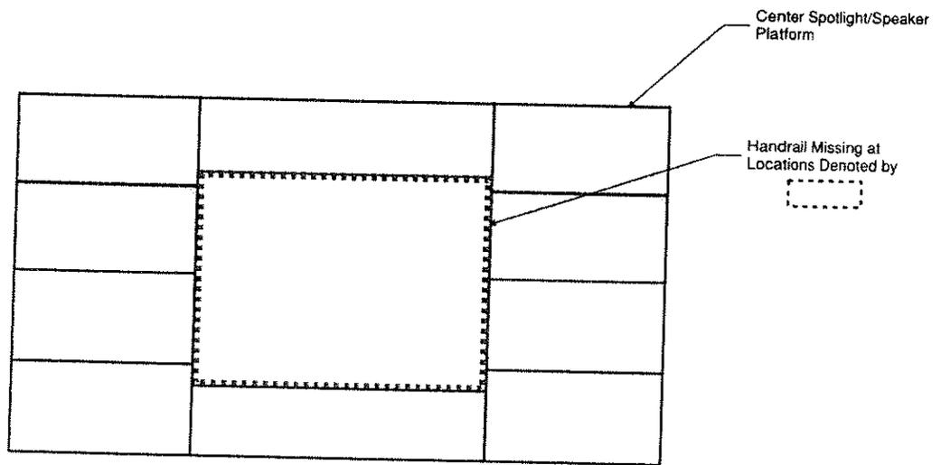
Figure 3a: Opening in the Center of the Spotlight/Speaker Platform
