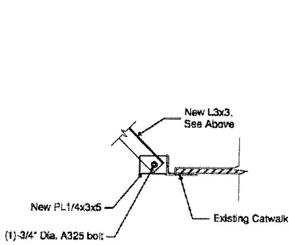
Figure 1b: Connection at Catwalk Angle
