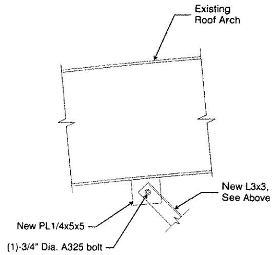
Figure 1c: Connection to Roof Arch
