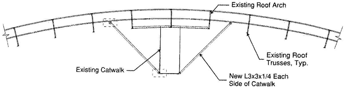
Figure 1a: Catwalk Bracing
