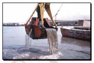
Figure 7. Mechanical dredge (clamshell bucket and barge).
