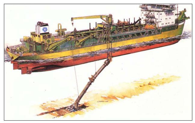
Figure 4. Hopper dredge illustration.
