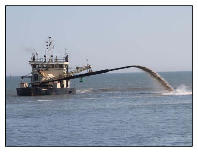
Figure 6. Side-casting dredge MERRITT.
