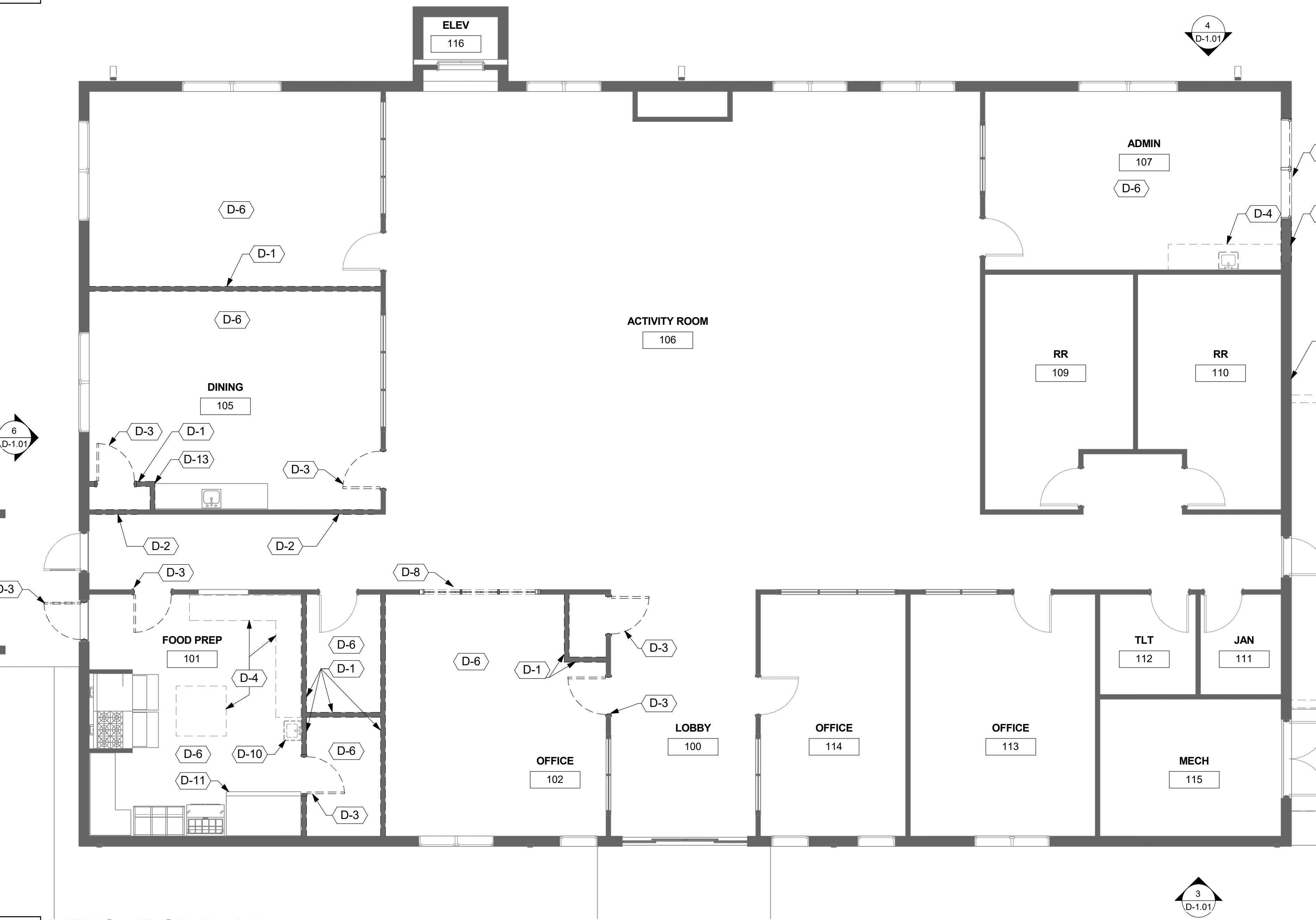
1 DEMOLITION PLAN SCALE: 3/16" = 1'-0"
