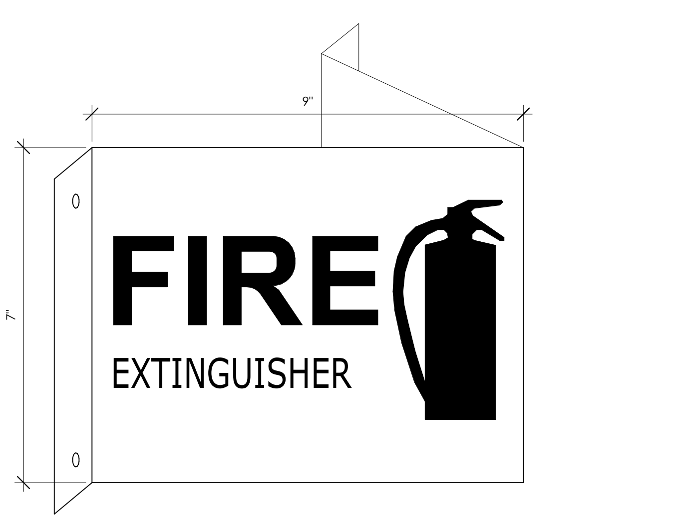
2 PROJECTING FIRE EXTINGUISHER SIGN SCALE: 6" = 1'-0"
