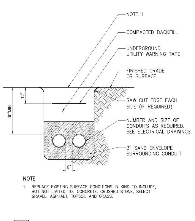
1 TYPICAL DIRECT BURIED CONDUIT(S) DETAIL - NOT TO SCALE
