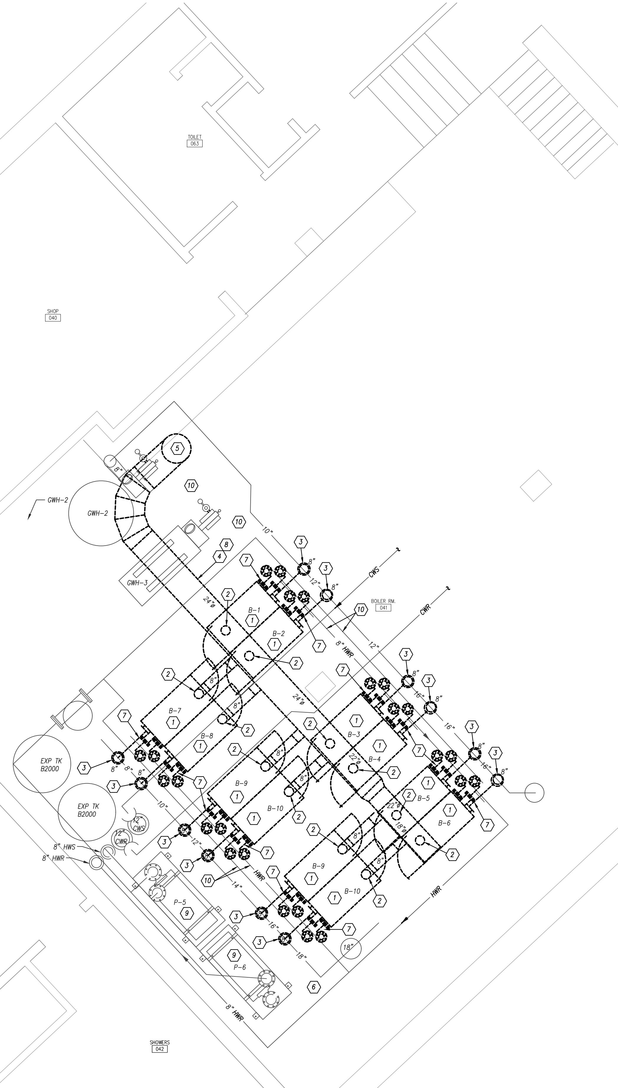
BOILER ROOM PLAN - DEMOLITION 1/4" = 1'-0"
