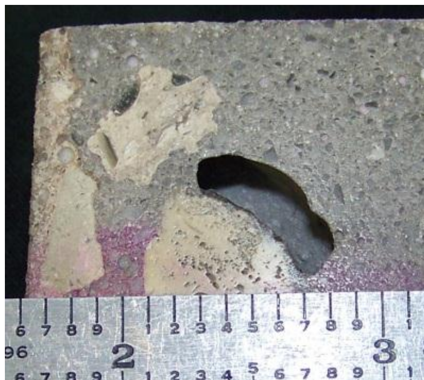
Photo 11 – Sample 2 – magnified view of entrapped air void.
