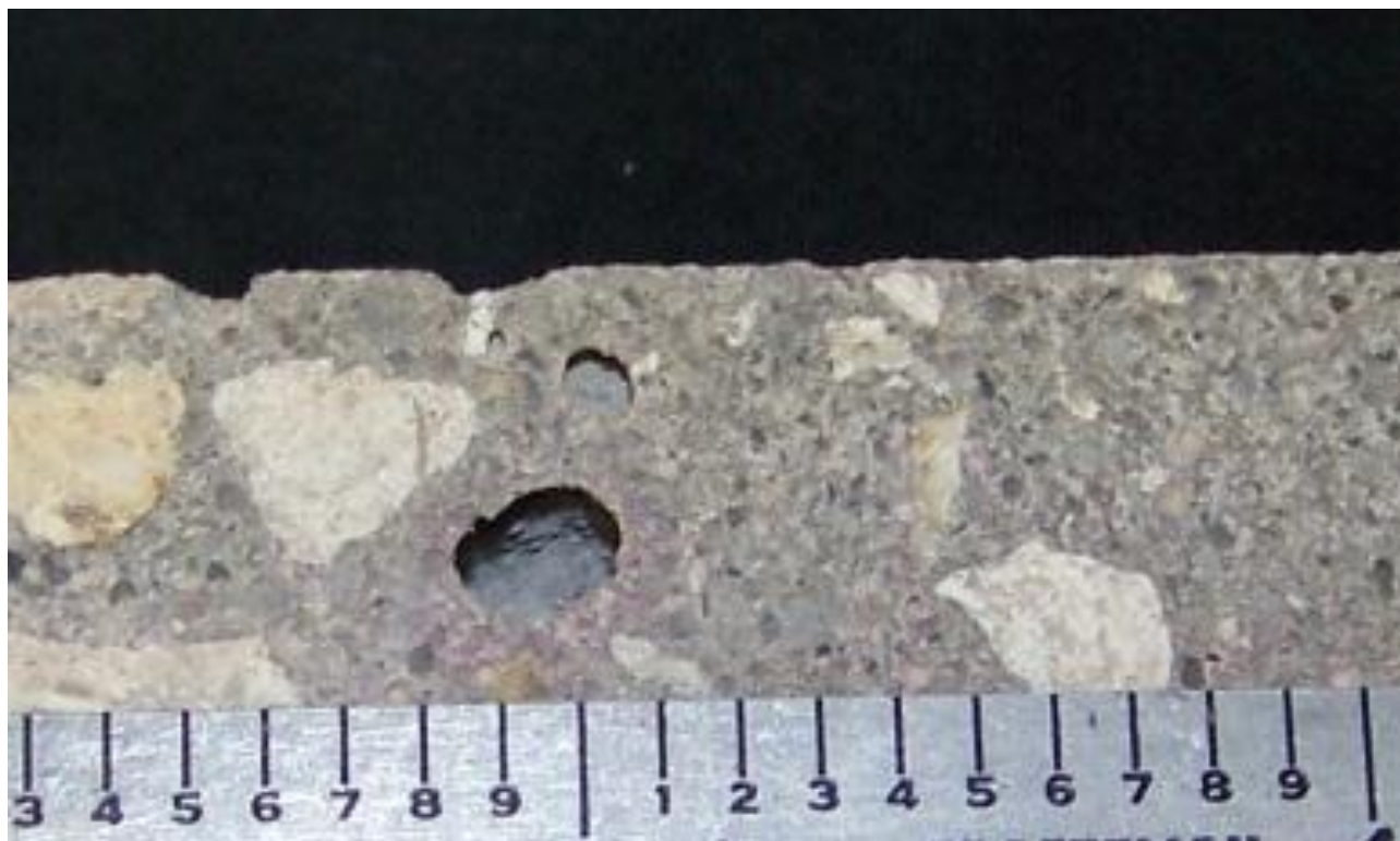
Photo 10 – Sample 1 – magnified view of entrapped air void.
