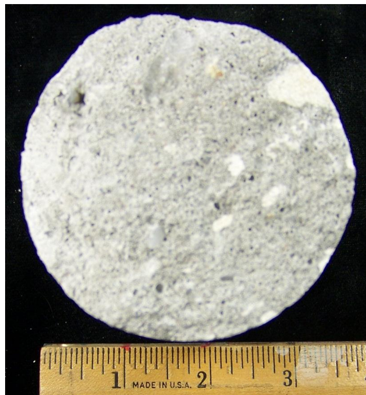
Photo 5 – Sample 6B – Inside fractured face (end).
