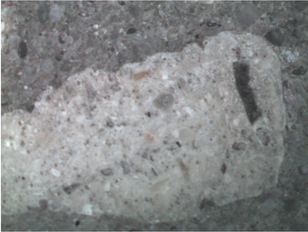
Photo 4 – Sample 2 – magnified view of typical coarse aggregate piece, note no signs of cement-aggregate reactions.
