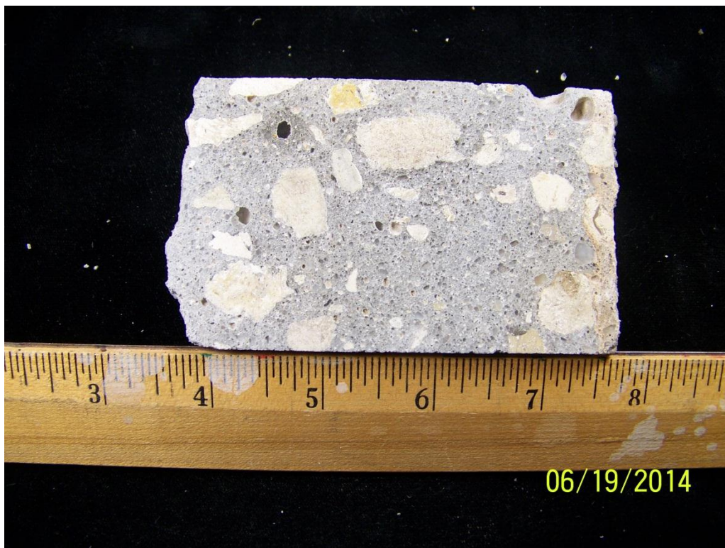
Photo 7 – Sample 6B – Polished surface of core..
