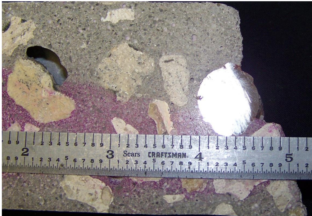
Photo 5 – Sample 2 – No. 6 reinforcing steel bar, located 2 \frac{3}{4} inch from surface. No evidence of corrosion noted on steel.
