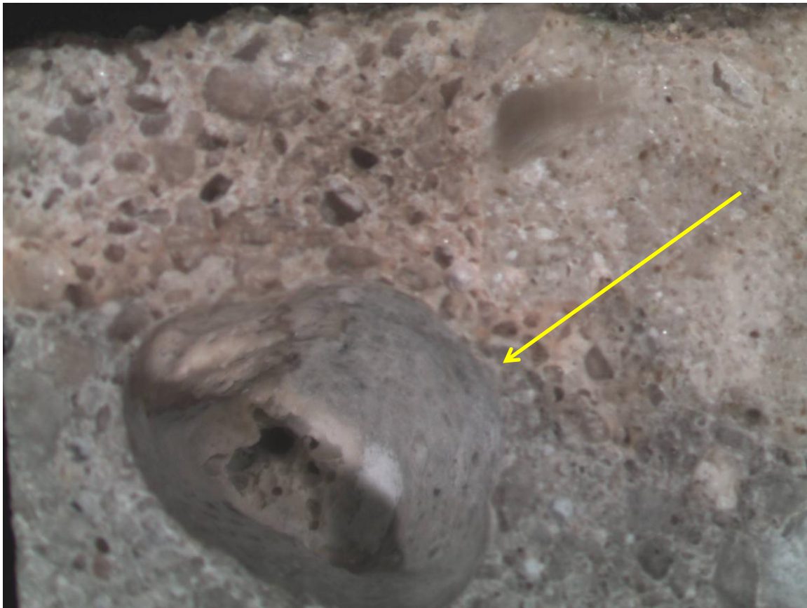
Photo 11 – Sample 2 – magnified view of entrapped air void near surface of core.
