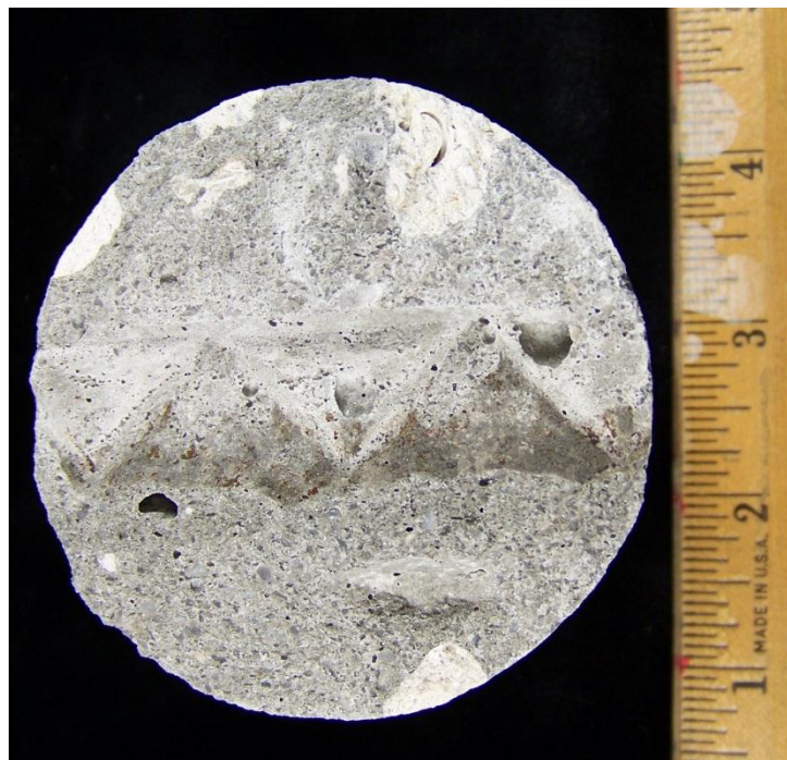
Photo 3 – Sample 3B – Inside fractured face (end) – note reinforcing bar impression.
