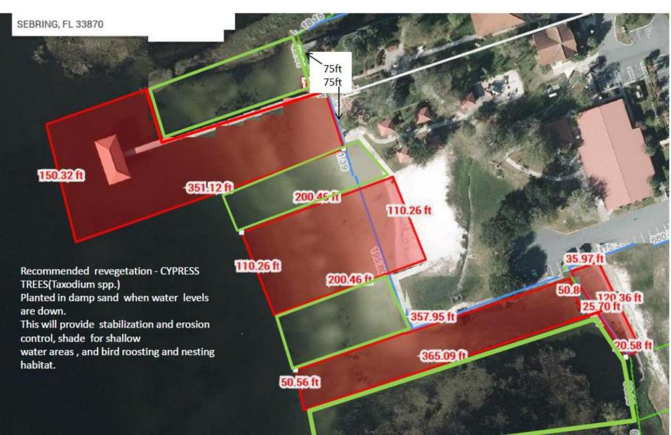
Hidden Beach Site Plan Access Corridor Lake Jackson Map not to scale Revegetation Zone City of Sebring Recommended revegetation -CYPRESS TREES(Taxodium spp.) Planted in damp sand when water levels are down. This will provide stabilization 110.23 ft and erosion control, shade for shallow water areas, and bird roosting 30ft and nesting habitat. 36ft 150 23 ft 150.13 ft 110.66 ft
